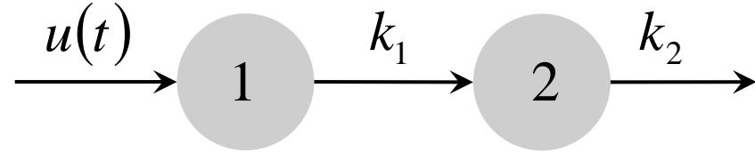
$$\begin{aligned} \frac{dq_1}{dt} &= -k_1 \cdot q_1 + u(t) & q_1(0) &= 0 \\ \frac{dq_2}{dt} &= k_1 \cdot q_1 - k_2 \cdot q_2 & q_2(0) &= 0 \end{aligned}$$
